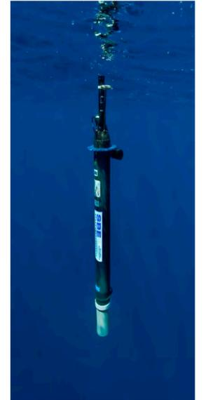
NAVIS BGC float 0028 (above) after deployment in the Mediterranean Sea. The float used in this study was equipped with and MCOMS and pH sensor. Photo by Christoph Gerigk.
