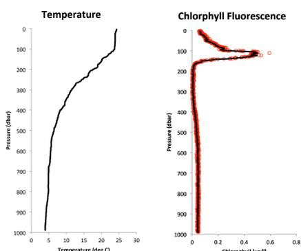
Temperature data (left panel) from both the transmitted and recorded data sets overlaid in the left panel demonstrates no effective difference between the two data sets.
