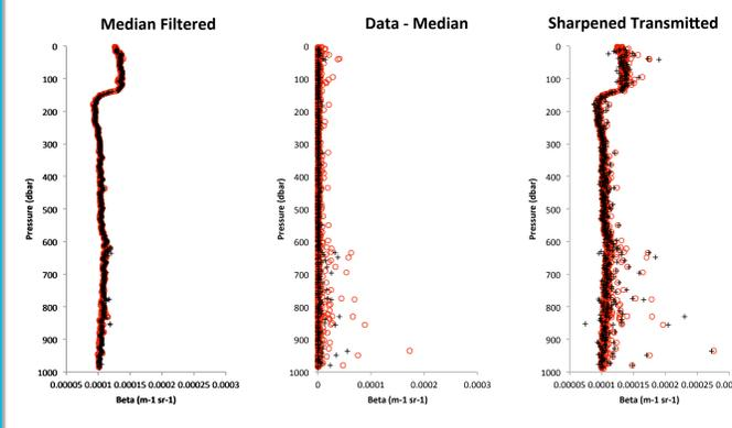
Applying a running median filter to both data sets (far left) generates coherence between both profiles. The residual data, assumed to be the large particles, again shows the undercounting in the transmitted data (middle). Using a sharpening algorithm (right), much of the recovered data can be generated from the transmitted data.
