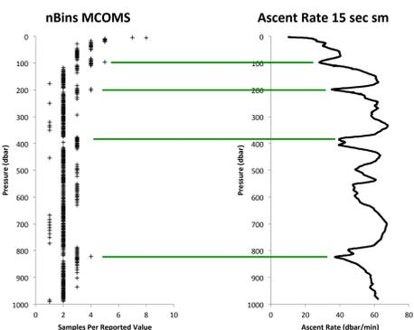
The Navis float's ascent rate modulates the number of subsamples within each individual transmitted bin. The horizontal lines connect the negative peaks in the ascent rate with the local increases in the number of subsamples per pressure bin. Since the ascent rate is a function of the density gradient, the float will collect more samples where the gradient is increasing.
