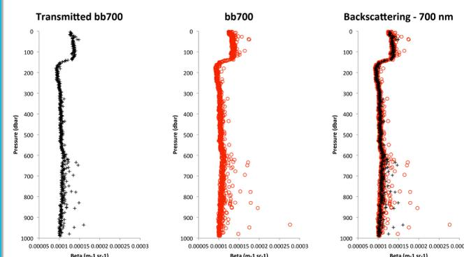
The transmitted backscattering data (far left), the recovered data (middle), and both data sets overlain (right). The recovered data demonstrates that the transmitted data smooths the variance in the recovered data. Assuming the 'spikes' represent relatively rare large particles, the transmitted data undercounts the large particles.
