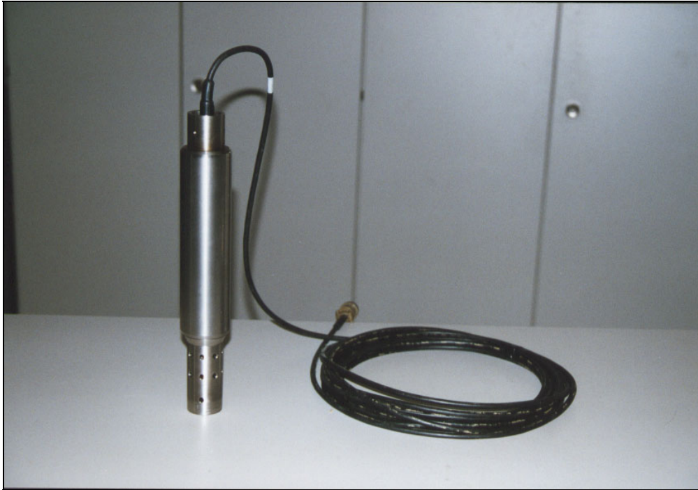
Figure 4 - Protection of the Sea Bird probes placed downstream of the turbines
